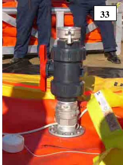
PICTURE 33: OPEN TOP “VENT” VALVE BEFORE FILLING
