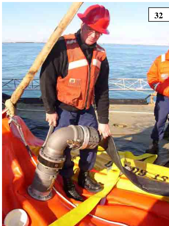
PICTURE 32: CONNECT FILLING HOSE TO THE SEA SLUG BEFORE DEPLOYMENT AND OPEN THE VALVE
