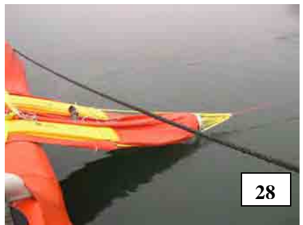
PICTURES 26 TO 31 LAUNCHING THE BLADDER (FCB-250 "100 m 3 ") FROM THE STERN OF A VESSEL
