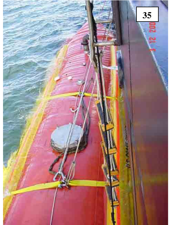
PICTURES 34 & 35: SEA SLUG MOORED TO SIDE OF THE VESSEL WITH THE “BELLY BANDS”
